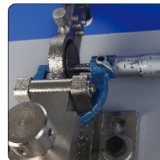
Lapping measuring surfaces of outside micrometer
