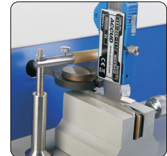
lapping measuring surfaces of caliper lower jaws
