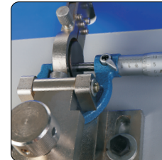
Lapping measuring surfaces of outside micrometer
