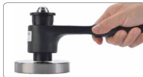
Hammer impact to apply test force
