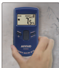
Measure concrete moisture
