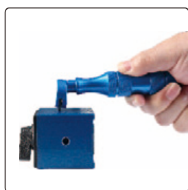
step 1: make grid cutting on surface
