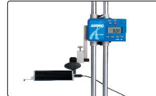
Working with height gauge
